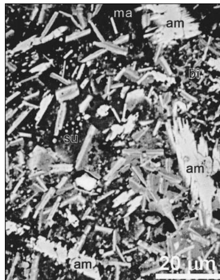
Figure 1. Backscattered-electron image of typical pseudotachylyte from Nason terrane. Sample consists of large, slightly dendritic crystals of amphibole (am); medium gray biotite crystals (bi); small, bright, blocky Fe sulfide crystals (su); and dark matrix with a calcic plagioclase composition (ma). Some of the small bright crystals (<1 \mu m) may be clinopyroxene. Most of the K in such samples resides in biotite. Sample N246-4b.
