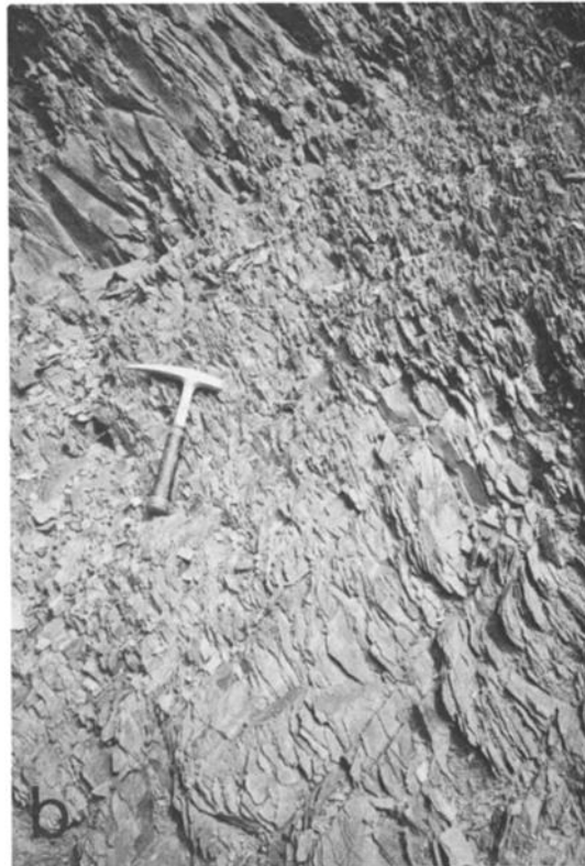
Fig. 3. Field photographs of (a) uncleaved Martinsburg Formation shale with bedding dipping 43^{\circ} to the north and (b) well-cleaved slate, with slaty cleavage perpendicular to bedding, dipping 65^{\circ} to the south.
