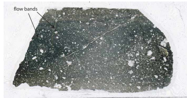
Fig. 9 Thin section of OU 74177 displaying flow banding (section length 50 mm).
